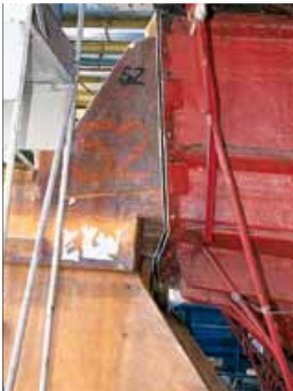
**An extension on the transom of the GB49 molds extends the hull out for the new GB52.**
